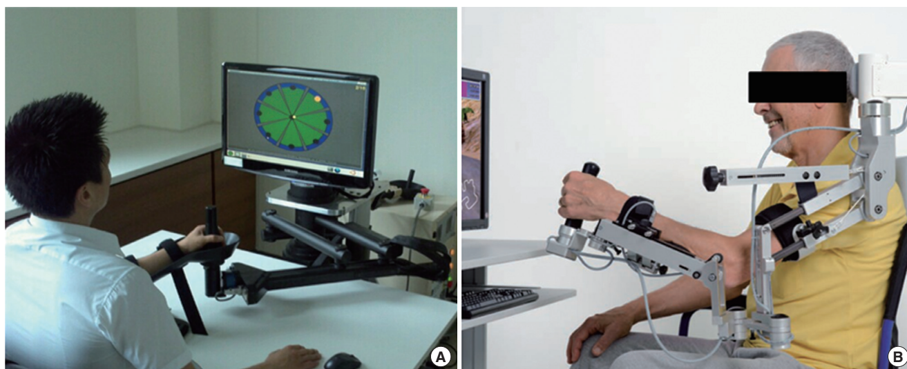
Figure 1. Examples of robotic devices for motor training (A) End-effector type (InMotion 2.0 Interactive Motion Technologies, Watertown, MA, USA), (B) Exoskeleton type (Armeo®, Hocoma, Switzerland).
